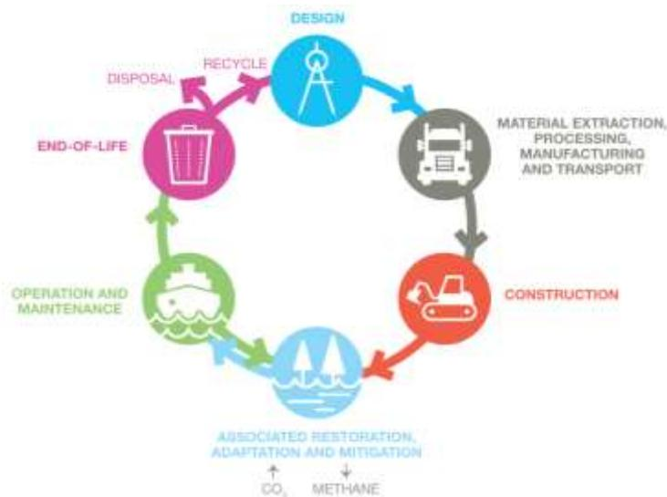
Figure 1: WG188 Carbon Management Life-cycle for Ports and Navigation Infrastructure and Projects
