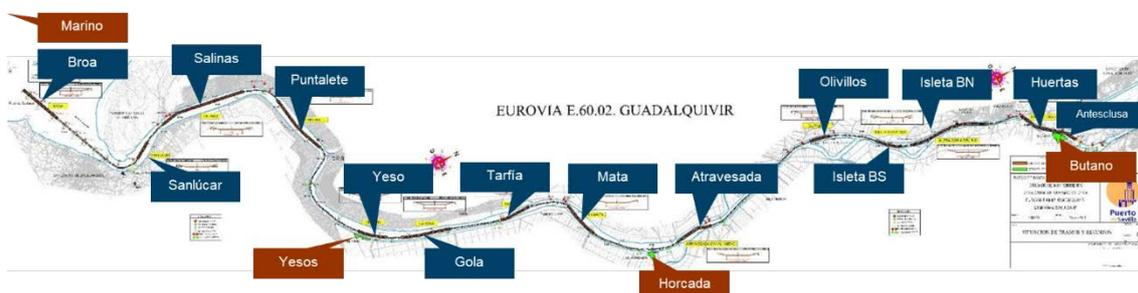
Figure 19. Historic sections in which the Eurovia Guadalquivir is divided for maintenance dredging. Source: Port Authority of Sevilla
