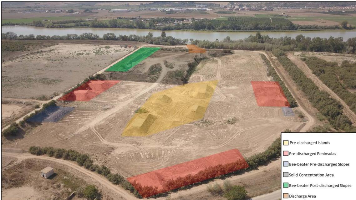
Figure 31. Final configuration of Butano Sector B after adaptation works.
