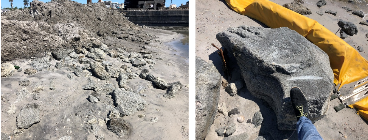
Figure 3. Coquina Encountered Within the Dredging Template Overdepth
