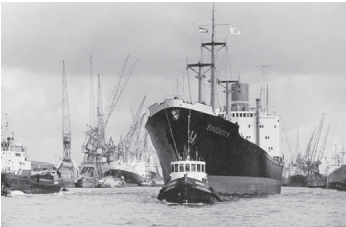
The general cargo ship was the work horse of the fifties and sixties. Then the container emerged and almost completely replaced general cargo. The many slim quay-side cranes were replaced by huge portal cranes to tranship containers.
