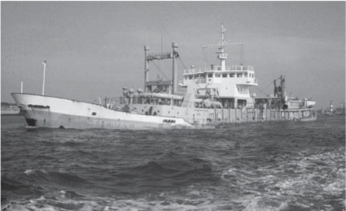
Gradually, the trailing suction dredger took over the dominant position from the bucket dredger. Suction dredgers were more flexible, had less down time at sea and were much more efficient and cheaper as their size increased.
