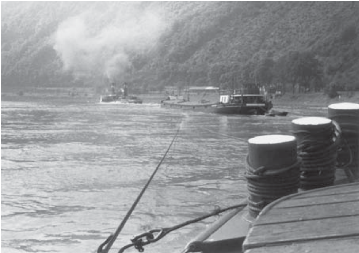
On the River Rhine, powerful steam paddle tugs towed barges up and down stream. The dimensions of such barges formed the basis for the 1954 European classification of inland waterways.
