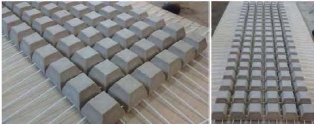
Figure 6: Articulated concrete mattresses (as modelled)
