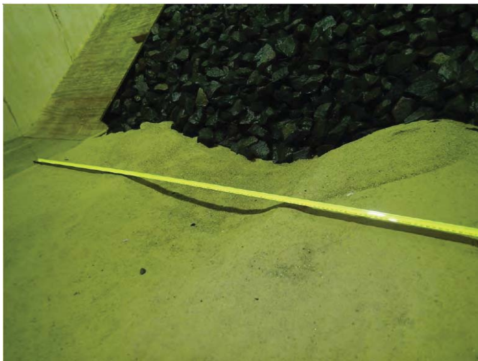
Figure 13: Photo of Test 2b scour hole formation
