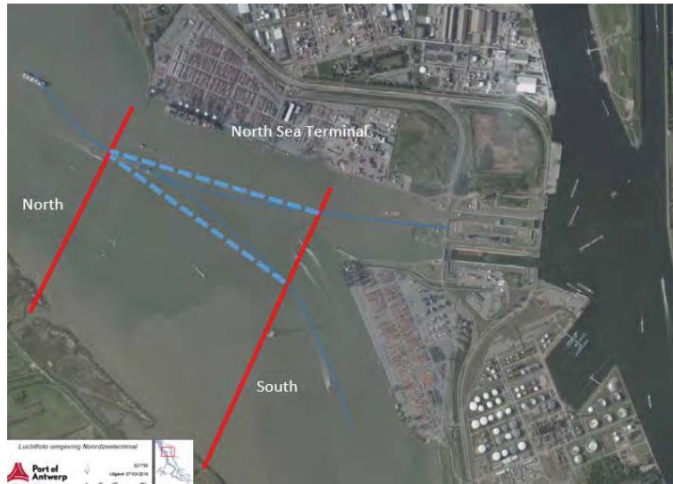
Figure 3-1 : Northern and southern measuring section and assumed straight trajectory. – image courtesy of Antwerp Port Authority
