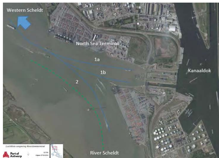
Figure 2-1 : Port Of Antwerp ; Location North Sea Terminal; Three examples of passing trajectories (blue) and edge of navigational channel (green dash). – image courtesy of Antwerp Port Authority
