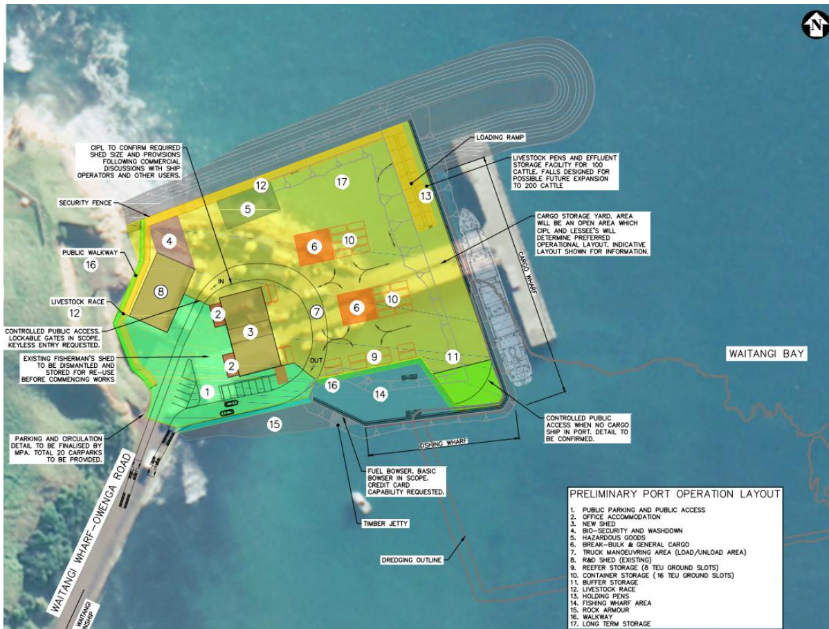
Figure 4 – Layout of the proposed Waitangi Wharf. Showing the key features relative to the existing situation. Note to reviewer – better quality image with readable text will be sourced.
