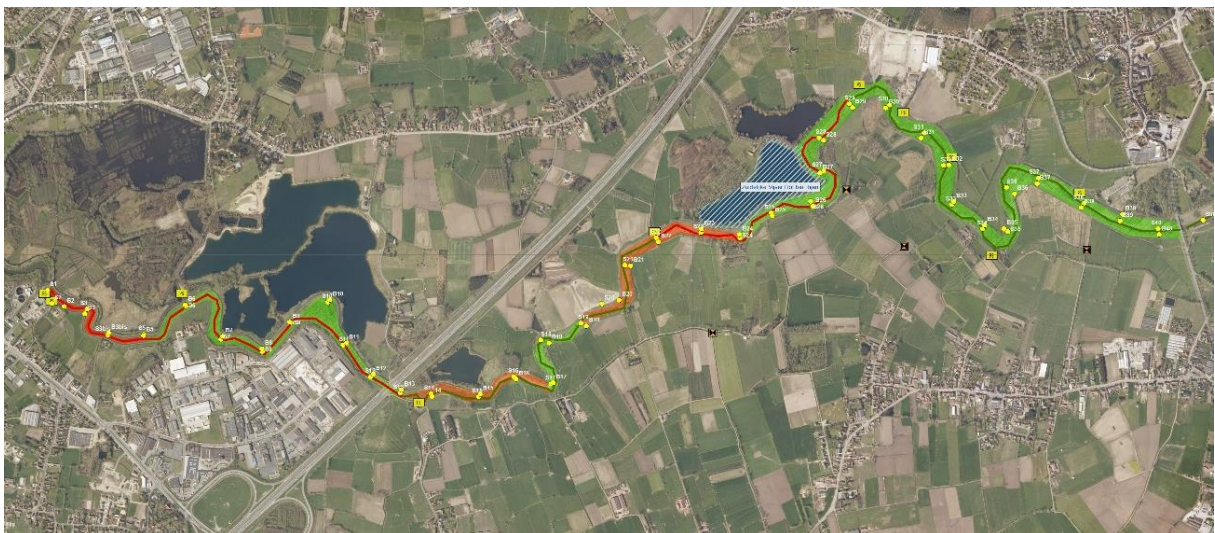
Figure 9: Map indicating exceedance of quality criteria for use of the sediment as building material, both in the river bottom (red line) and the slopes (orange area)
