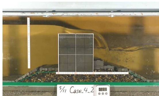
(b) Test against Tsunami in wave flume
