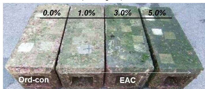
Figure 11 : Monitoring condition of blocks taken from underwater after 8 months
