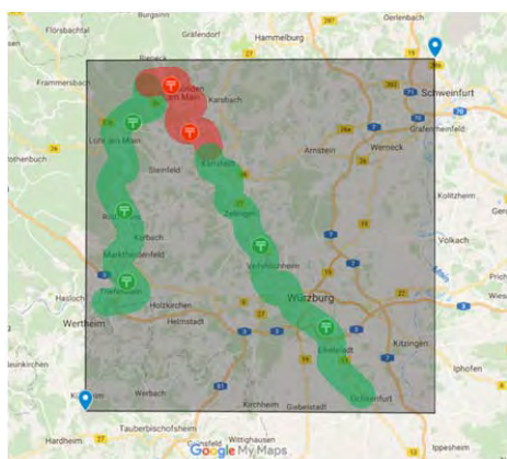
Figure 5: Test bed Main River with additional AIS land-based transmitting on new VDES frequency channels (green) and area for GSM connection (red); Dark grey, regional area for frequency channels 2025 and 2026
