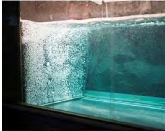
Figure 6: Closely packed air curtain in the laboratory (from Keetels et al., 2011)
