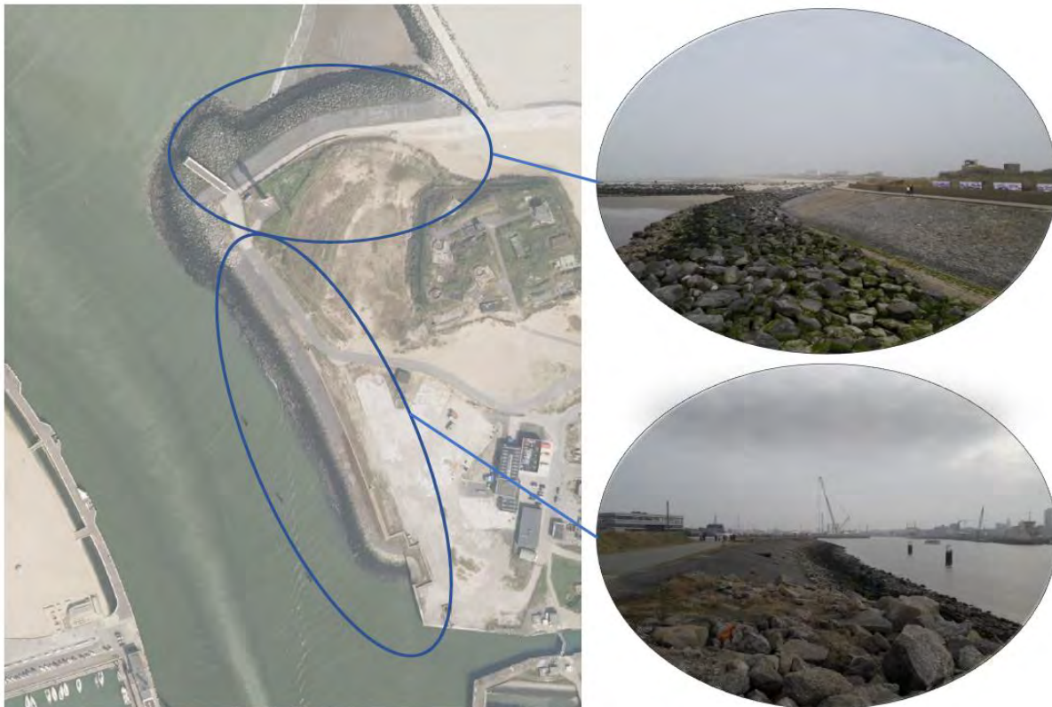
Figure 4: 'Halve Maan' site as it is today, with existing dike and revetment parallel to entrance channel
