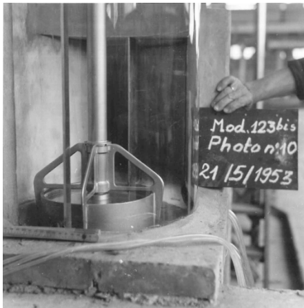
Figure 15: Scale modelling of Marchienne lock cylindrical valve. (a) Model (LRH, 1954); and (b) measured head loss parameter K = \zeta/2gA .
