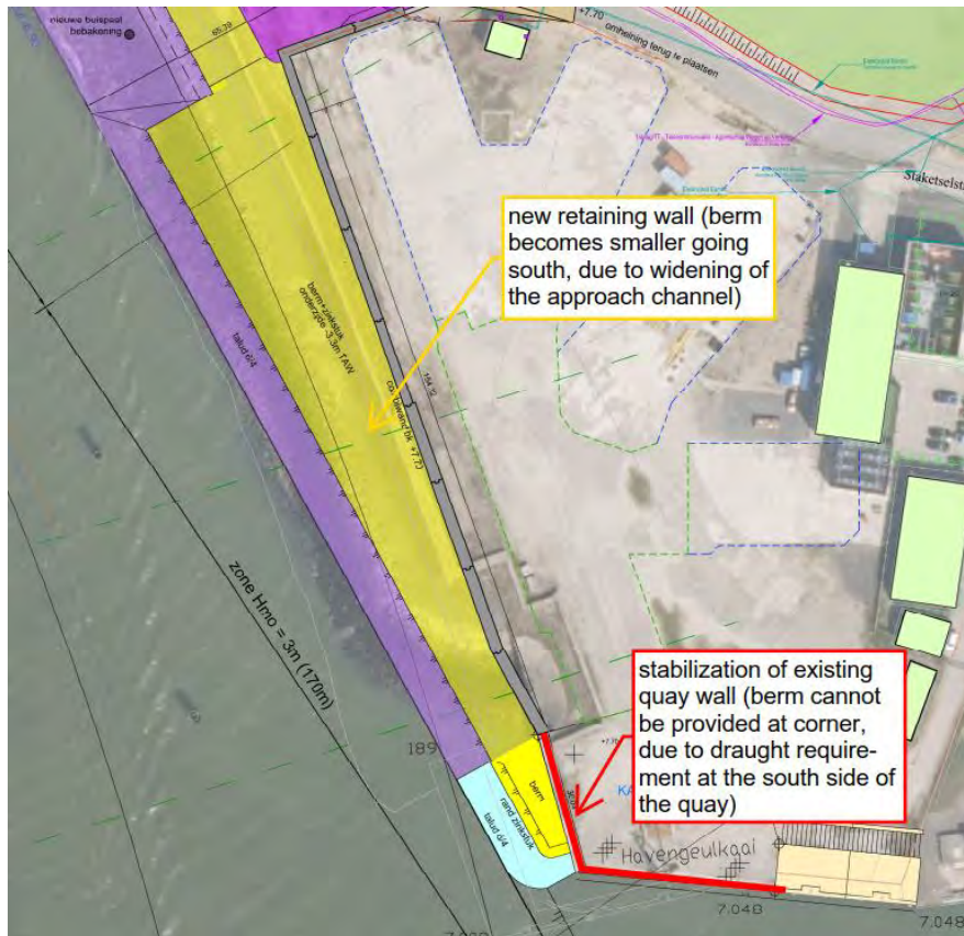
Figure 13: Design for middle and southern project area (retaining wall and quay wall stabilization)
