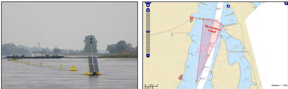
Figure 3: Cable ferry at the river Elbe, virtual caution area while the ferry is crossing
