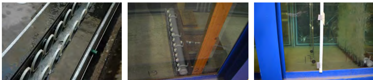
Figure 7: Overview of scale model set-up by Van der Ven and Wieleman (2017): (a) bubble caps as built in the Krammer recreational lock; (b) caps used for the scale model of the bubble screen; (c) overview of the EMS instruments and bubble screen during a test condition
