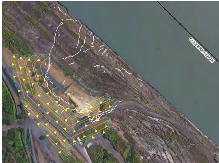
Figure 14: Excavation Layout at Old Lirio Slide
