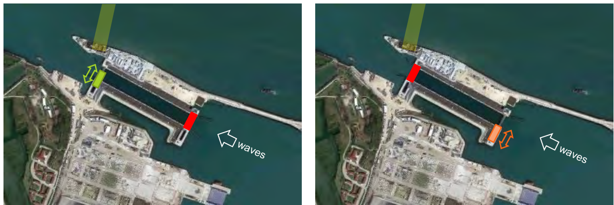
(a) If the sea side gate is closed, the lagoon side gate is protected and can be operated (b) When the sea side gate is opened or absent during acqua alta , the lagoon side gate must be closed and anchored.
