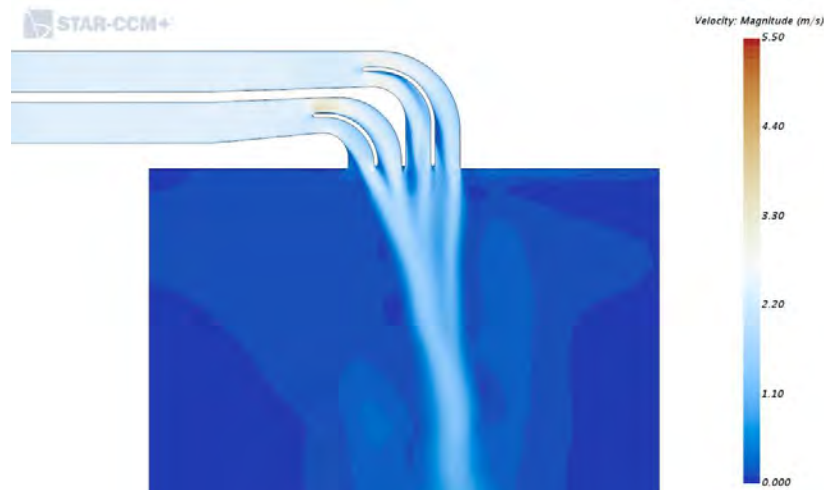
Figure 8: Top view of velocity field for the outflow at the outer harbor when emptying the lock
