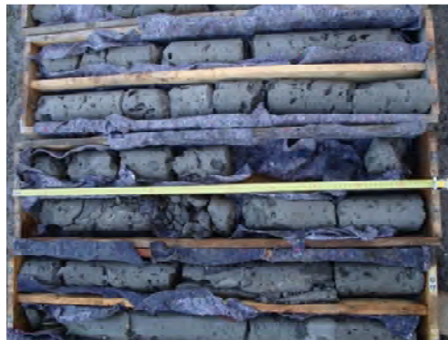
Figure 13: Core drill holes of the jet-grout columns at De Gerlachekaai with clearly visible clay inclusions
