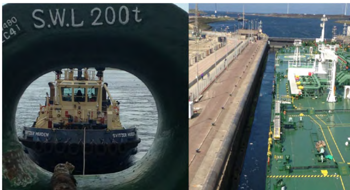
Figure 4: Left panel: View through a fairlead on a tugboat that measures the longitudinal force; right panel: Aframax tanker 'Densa Crocodile' in the North Lock during the measurement campaign.
