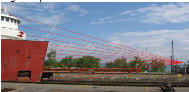
Figure 7: Laser Scanner to spot vessel into lock
