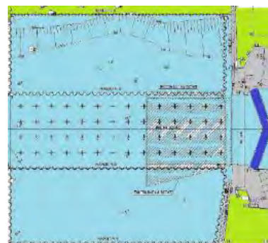
Figure 7: Closure period 1 - View of the two small sheet pile cofferdams
