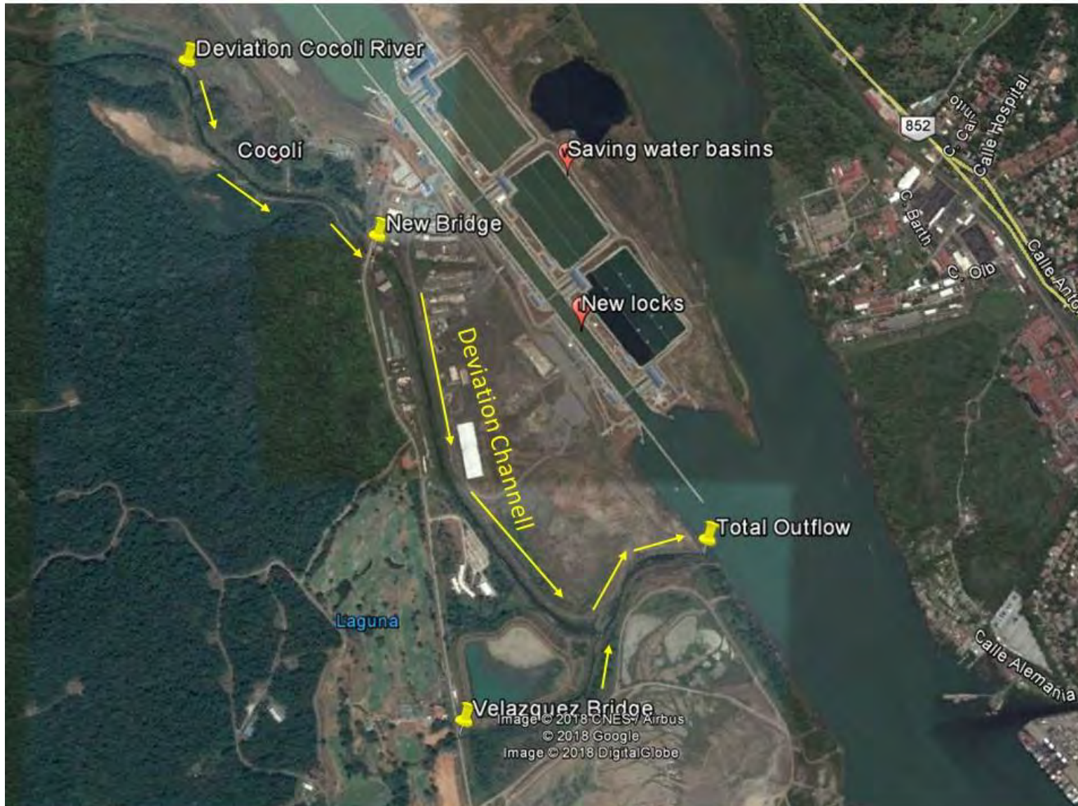
Figure 29. Image of the Cocoli river deviation channel and the new locks of the Pacific side.
