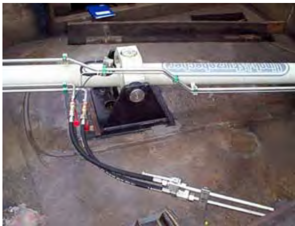
Fig. 16: Supporting of gate cylinder for quick replacement
