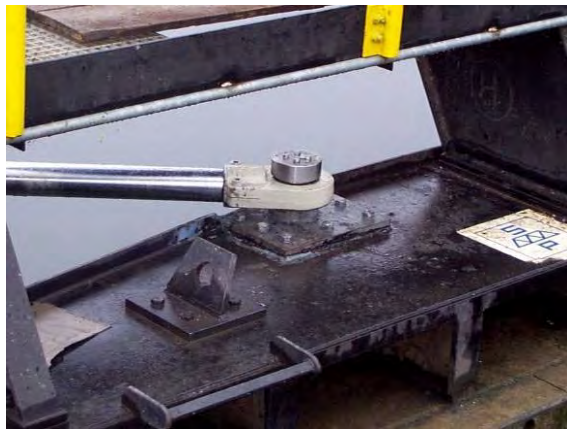
Fig. 18: Quick connect linkage of cylinder to a miter gate
