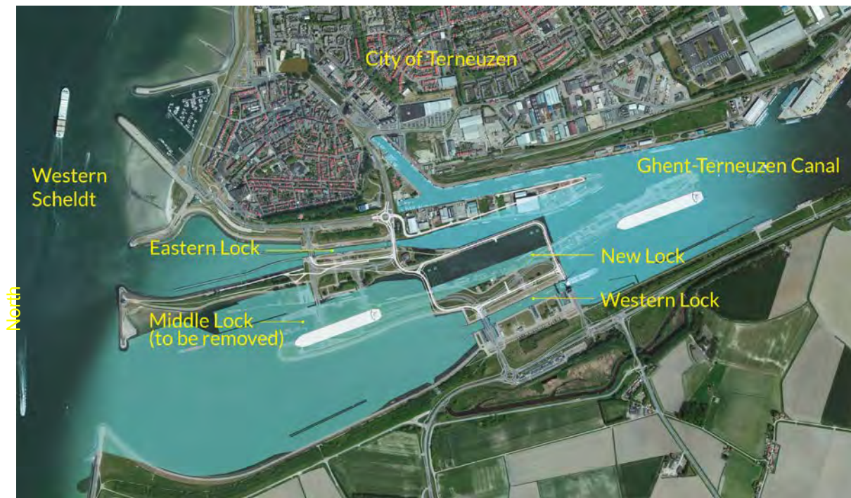
Figure 3. Project New Lock Terneuzen, with indication of the existing locks, the new constructions (black) and constructions to be removed (transparent)
