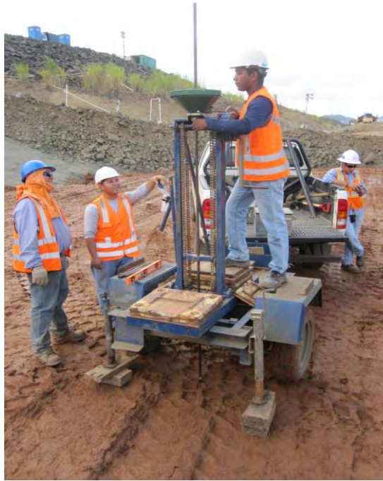
Figure 12. Vane shear testing of compacted core material
