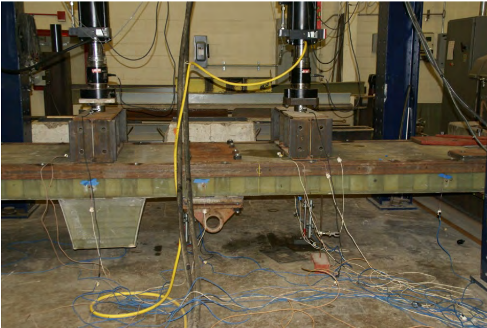
Figure 6: Flexure Test of Prototype FRP Wicket Gate
