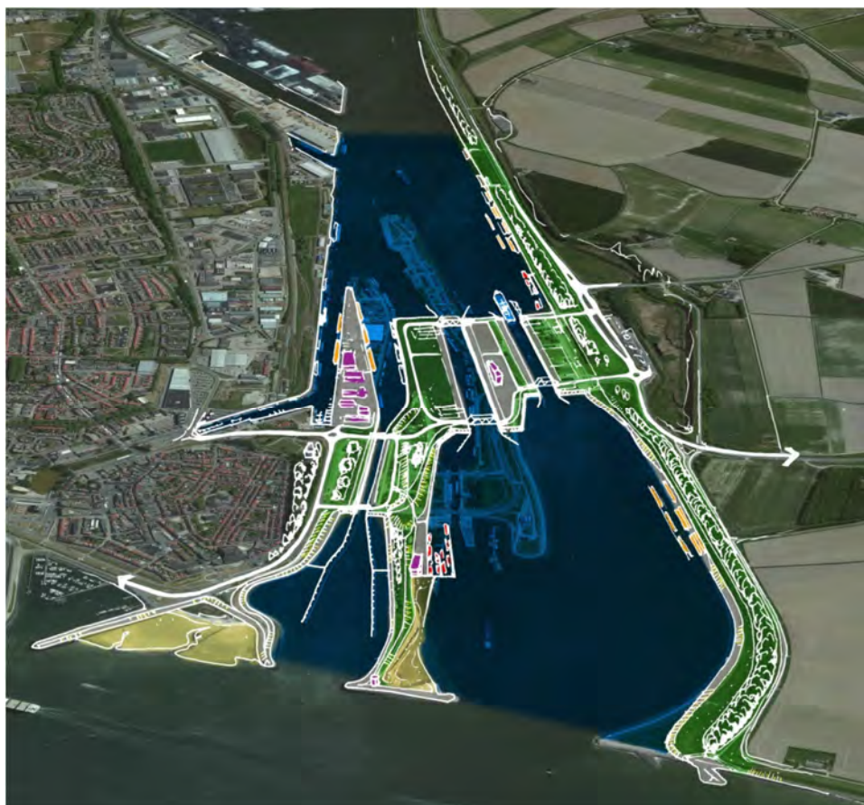
Figure 6 : sketch of the lock complex at Terneuzen. The New Lock will be constructed centrally in the complex and will replace the original Middensluis (VNSC, 2015)
