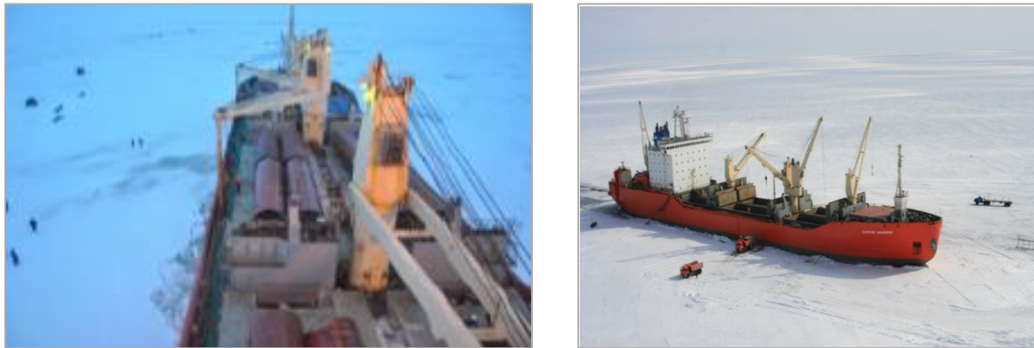
Figure 4: Unloading on ice with the multipurpose vessel SA15, offshore Sabetta (courtesy TOTAL)
