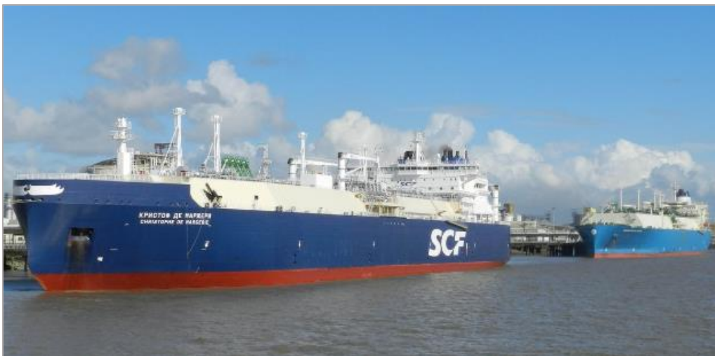
Figure 25: Trans-shipment at Montoir de Bretagne between an Ice-breaking LNG Carrier and a conventional LNG Carrier Courtesy of Nantes Saint Nazaire port
