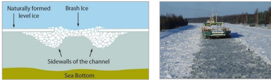
Figures 5: The formation of brash ice studied using ice breaker in a channel
