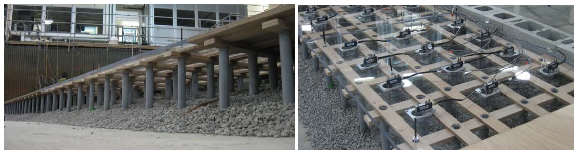
Figure 6. 1/30 scale model of deck-on-pile structure fitted with pressure plate sensors.
