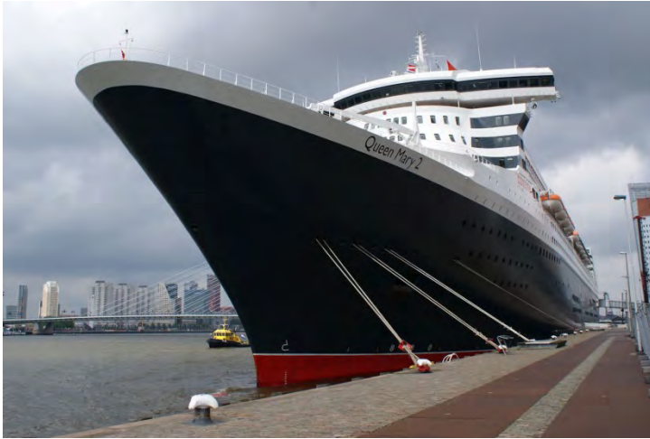
Figure 3. Parallel mooring lines in Rotterdam (photo Marco Alpha Fotografie)
