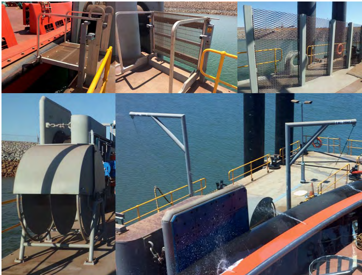
Figure 8: Operability features (clockwise from top left): access brow lowered, access brow raised, snapback guards, mooring line hangers, cyclone mooring line reels
