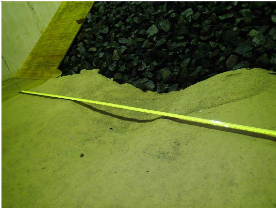
Figure 13: Photo of Test 2b scour hole formation
