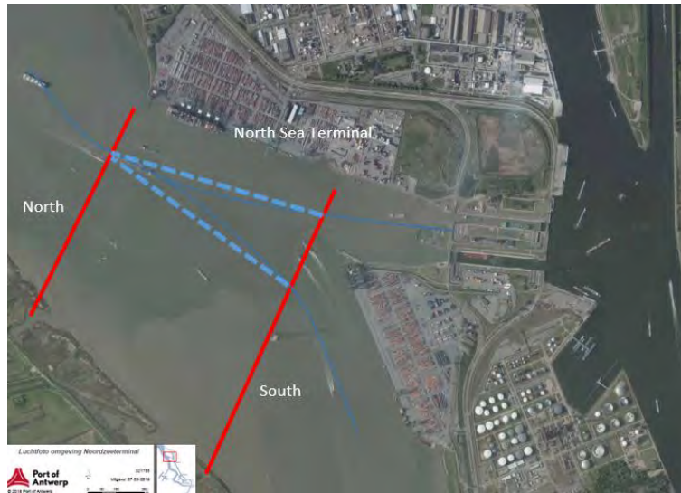
Figure 3-1 : Northern and southern measuring section and assumed straight trajectory. – image courtesy of Antwerp Port Authority
