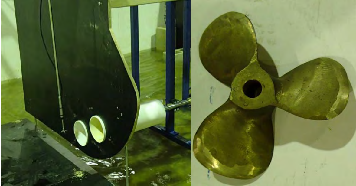
Figure 5: Bow thrusters installation with ADV probe (left) and view of a propeller used for a bow thruster (right)
