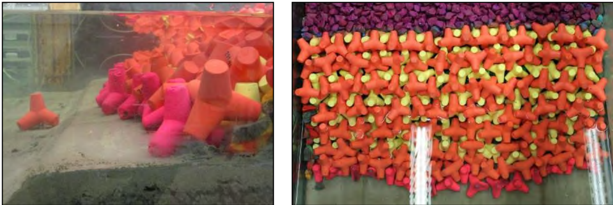
Figure 6 – Displaced toe and slumping of breakwater armor.
