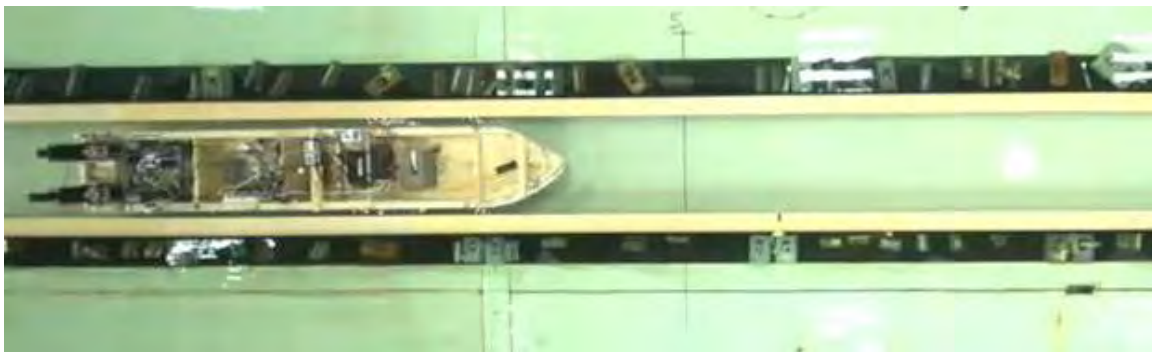
Picture 4: Model test of MS Midnatsol in the tunnel/channel
