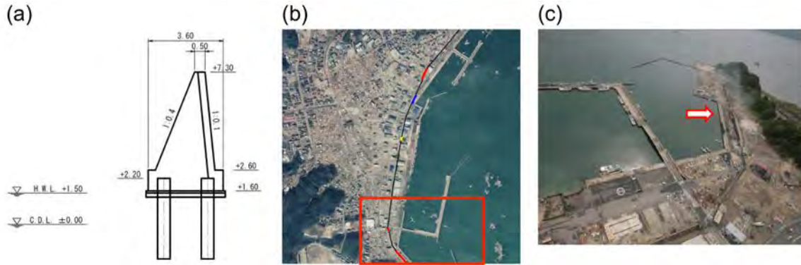
Figure 1: (a) A cross-sectional view of tsunami-affected seawall, (b) Example of seawall position (black-colored line). The red-colored line indicates the position of tsunami-affected seawall whose construction is similar to (a), and (c) Aerial photograph of the red-colored box area in (b). The arrow indicates a tsunami-affected area. (From the website of National Research Institute of Fisheries Engineering, Japan)
