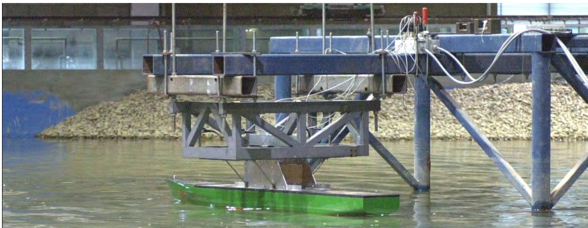
Figure 3: detail of moored ship held captive in the scale model (open water reference tests).
