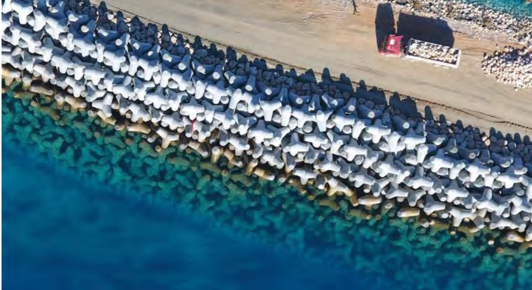
Figure 14. Prototype Tetrapod placement pattern
