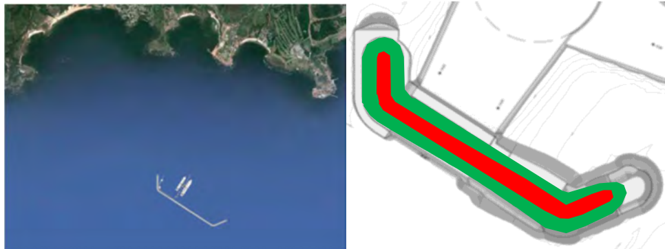
Figure 1: Location of the project (left) and approximate layout of the required scour protection layer (right): breakwater in red; scour protection layer in green.
