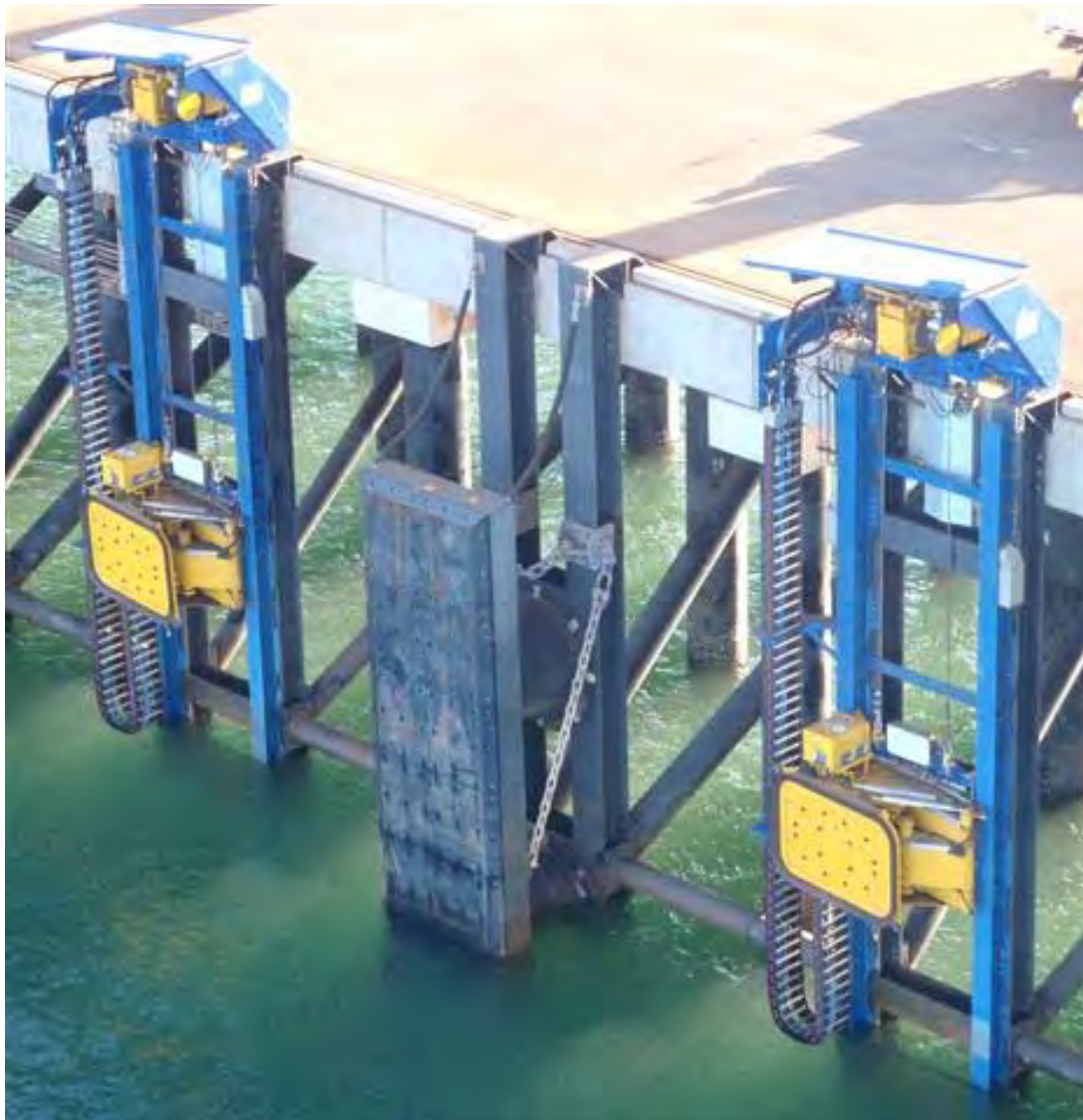
Cavotec MoorMaster™ MM200C 17 system installed in Port Hedland
