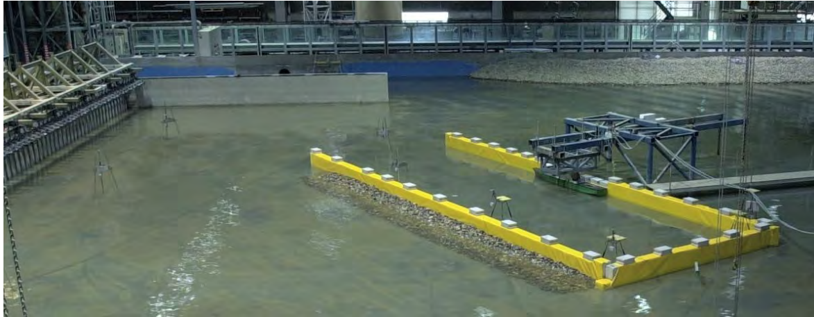
Figure 2: overview photo of a moored ship in a schematic representation of a harbour basin in the large directional wave basin of Deltares (the photo shows only a part of the basin).
