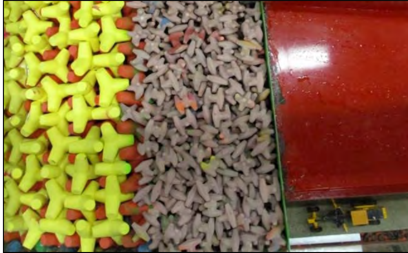
Figure 10. Overhead view of the breakwater crest with a 12.8m crest width and a Core-loc armor layer.
