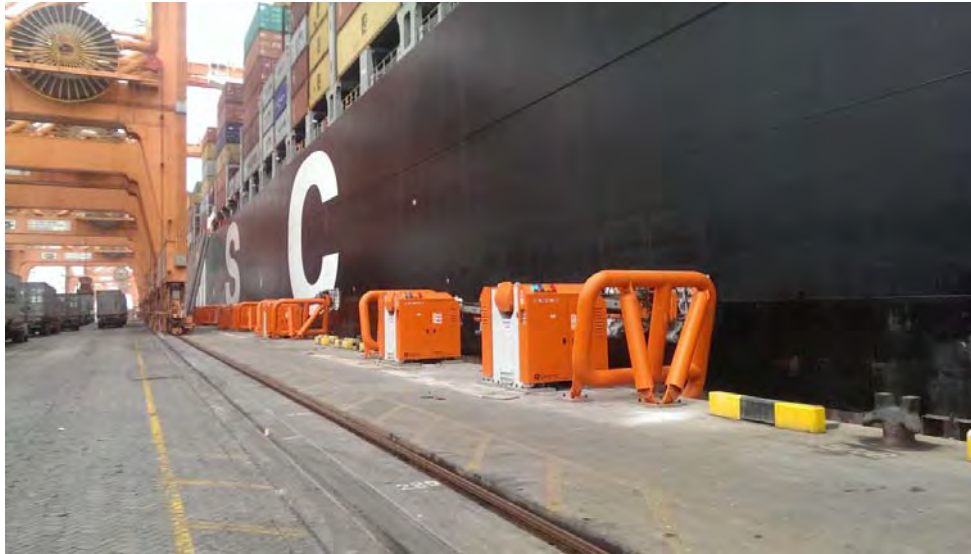
Cavotec MoorMaster™ MM400E 15 system installed in the Port of Salah
