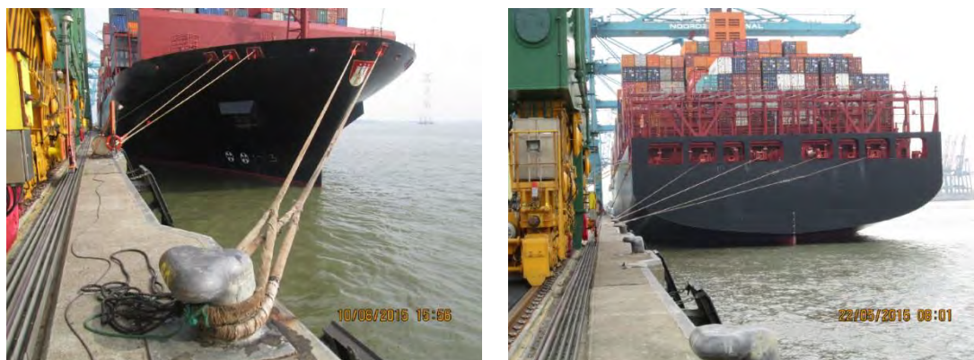
Figure 5-1 : Typical mooring configuration of moored 13000 TEU container vessels at North Sea Terminal, using 12 lines. – images courtesy of Antwerp Port Authority
